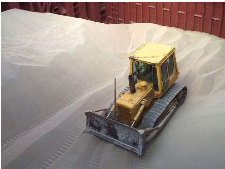
Trimming of cargo must be done with care
