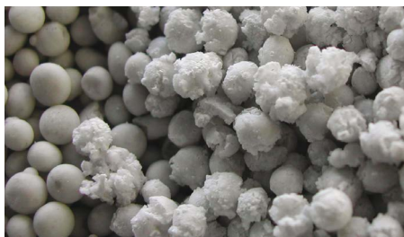
Distintegrated fertilizer due to water absorption
