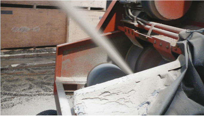
Avoid use of grain trimmers; fines formation will occur due to impact.
