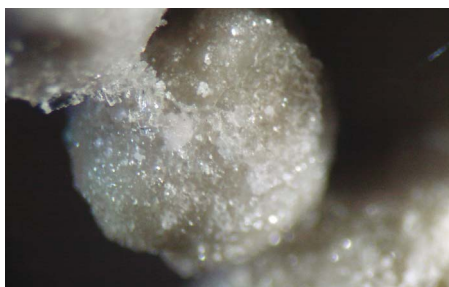
Crystal bridges between fertilizer particles cause caking
