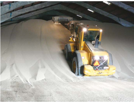
UNACCEPTABLE driving into pile
