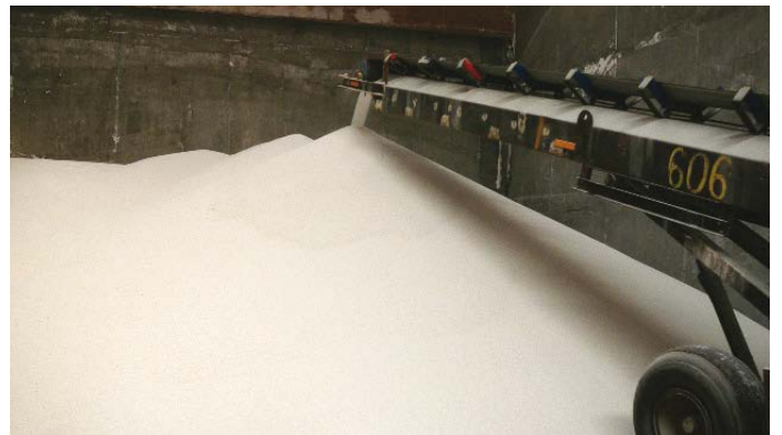
Moving regularly the tipper will avoid excessive segregation of the product.
