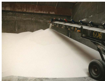
Good practice: moving the tipper to avoid segregation
