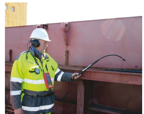
Testing for leaks by ULD
