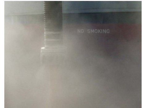
Excessive dust during loading vessel
