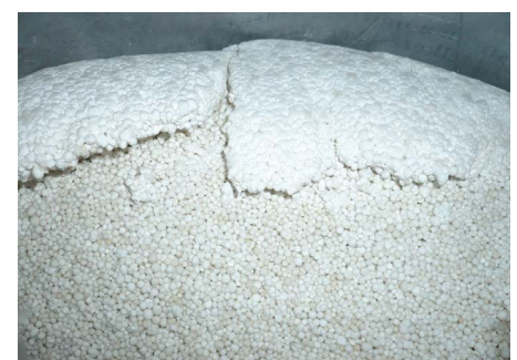
Thermal cycling leading to disintegrated product in the top layer of stored product
